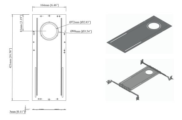
New construction housing plate for Round Gimbal Downlight
