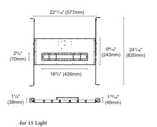
New Construction Plate for Trimless
